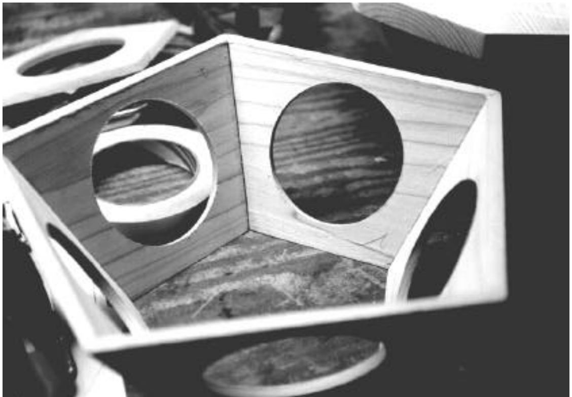
Figure 2. Images of the enclosure under construction, before insertion of the individual speaker enclosures. 7
