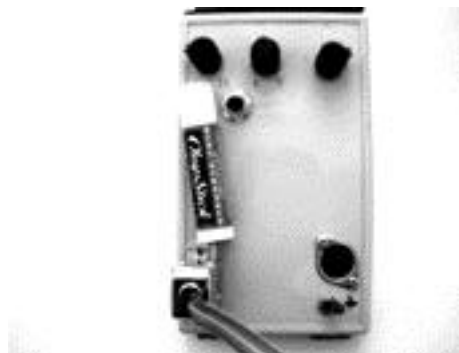
Figure 8. R-Bow belt-mounted computer (with ChapStick for scale)
